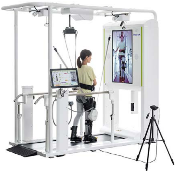
Toyota WelWalk WW-2000 Rehabilitation for patients with lower limb paralises
